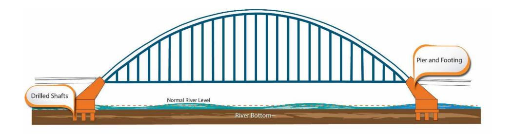
239 drilled shafts7-10' diameter20-30' depth
