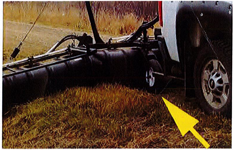
Gauge wheel keeps the boom at correct height to control drift
