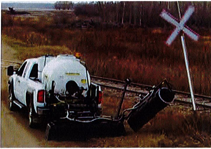
Boom break away with auto reset extends boom life, sprays more miles all day long.
